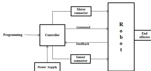
Figure 2: Block Diagram of General Purpose Robot
